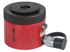
The BMLL-series is a design that features a threaded piston rod and lock ring. When the lock ring is screwed down and engaged with the cylinder body, the load can be held mechanically for extended periods. These cylinders are ideally suited to bridge construction and maintenance and jacking applications requiring safe extended load holding. All BMLL-Series cylinders feature a hard chrome bore for
